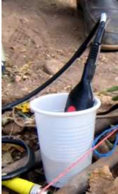
Figure 7 – A prototype dielectric tensiometer (DT160, Delta-T-Devices, UK) used in Turkey case study on cucumber, shown while wetted prior during installation.
