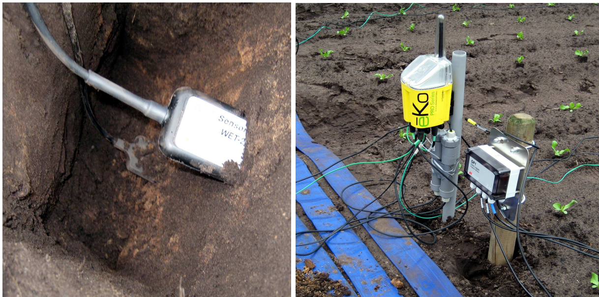
Figure 2 – A WET-sensor (Delta-T-Devices, UK) installed in the rooting zone at 15 cm and a 5TE (Decagon, US) installed underneath the rooting zone at 30 cm depth, both to measure water content, EC and temperature (left); a wireless sensor network (eKo, Crossbow, US) and irrigation controller (GPI, Delta-T Devices, UK) installed just after planting Iceberg lettuce in a Dutch case study.
