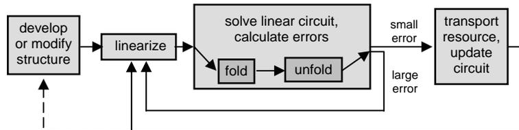
**Figure 7.** Phases of simulation. Each phase corresponds to an L-system derivation step. The L-system string is scanned from right to left in the folding phase, and from left to right in the remaining phases
