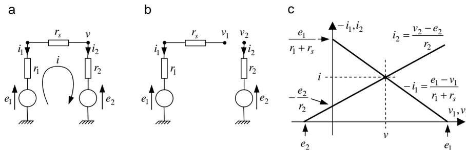
**Figure 5.** Graphical solution of a simple circuit. The circuit (a) is divided into two parts (b), represented by straight lines in the voltage-current plane (c). The solution to the circuit (a) corresponds to the intersection point ( $i, v$ ) of these lines
