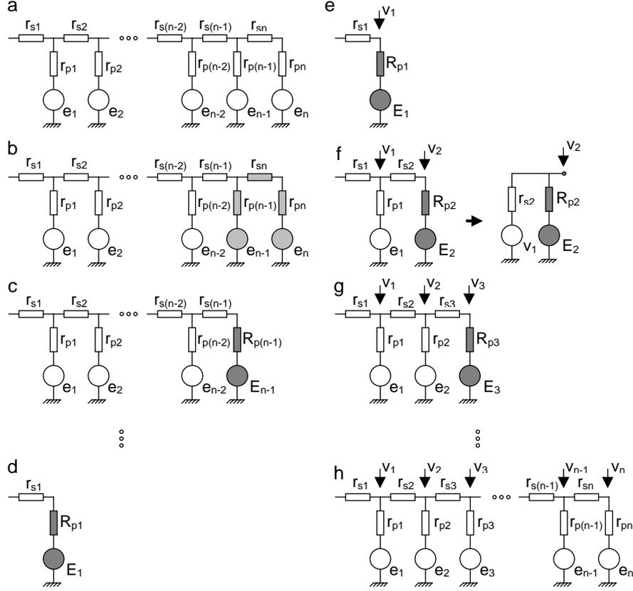
**Figure 3.** Solving a ladder circuit by a sequence of folding (a-d) and unfolding (e-h) operations. The dots between figures c-d and g-h indicate a continuation of the folding and unfolding processes. Down arrows labelled  $v_1, v_2, \dots, v_n$  indicate node potentials, computed one after another as the circuit is unfolded
