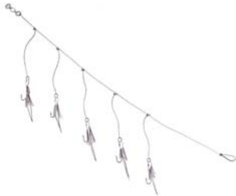
Figure 2.6. Feather paternoster with 5 hooks for mackerel (left) and herring paternosters (right).
