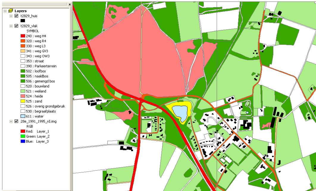
a: Top10Vector file with colour layout according to the top25 legend (part of mapsheet 28E)
