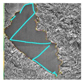
The trajectory traveled on the Lake is depicted in the figure to the left in blue. The mean depth turned out to be 2.16 ( $\pm$  0.62) m.
