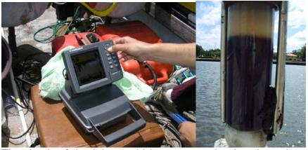
The depth of the lake could be measured using the echo sounder (left panel), unfortunately not the thickness of the sediment layer because of its composition. Some indication could be obtained from core samples (right panel).
