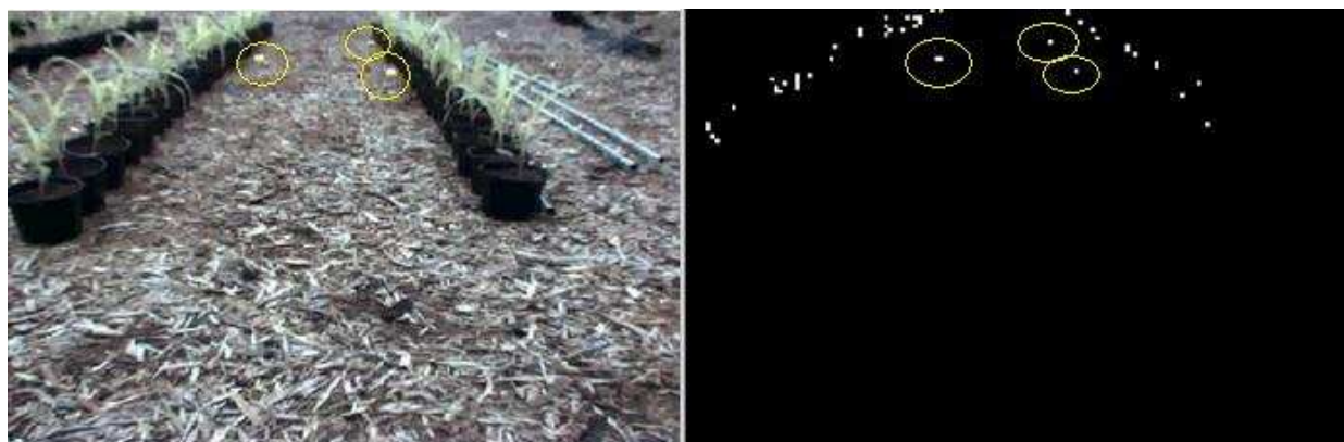
Figure 6: Test case scenario (left image) where we were looking for green plants and yellow referential objects. The result of image segmentation is shown on the right.
