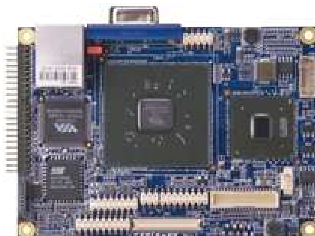
Figure 2: An embedded computer - VIA EPIA PX10000 (size: 10 x 7.2 cm).
