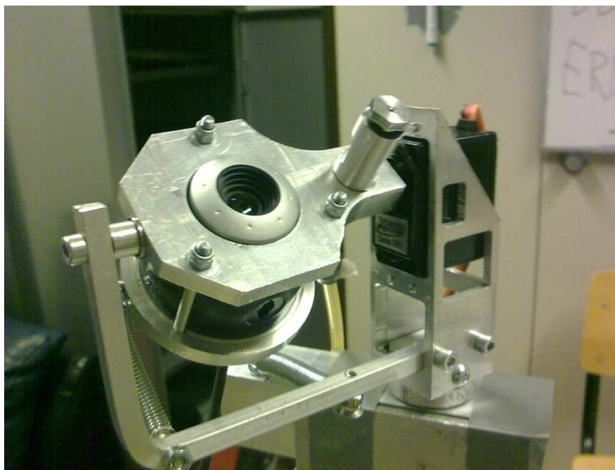
Figure 11: The webcam setup. The panning servo is mounted below the aluminum frame, inside the beam. Springs are attached to counteract the play in the servos.
