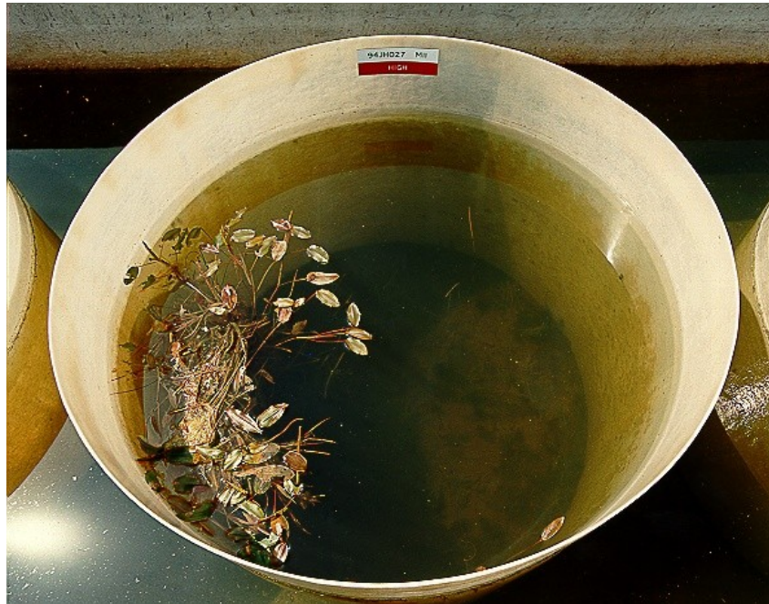
Figure 4: A 1 m 3 pond microcosm test system used for European regulatory purposes at Jealott's Hill Research Station, Bracknell, Berkshire, UK in 1994.
