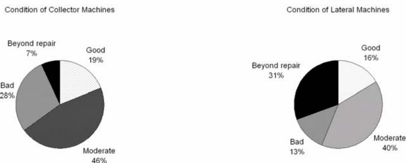
Figure 5.9 Operational research on the performance of drainage machines greatly improved the planning: example of operational research in Egypt [142].
