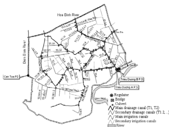
Figure 6.7 The lay-out of drainage systems in the Red River Delta is complicated (Example Trieu Duong area).
