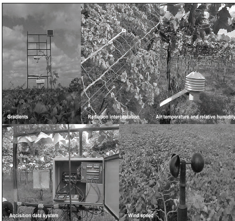
Figure 4.3 Measurements of net radiation over and under canopy; air temperature and relative humidity; wind speed; and automatic data collection in Bowen ratio system of table grape.
