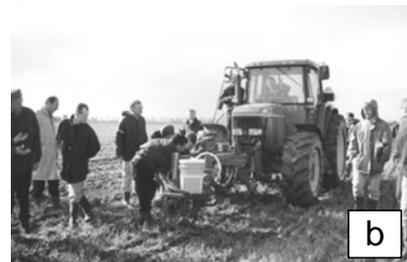
2000–01 Fourth generation prototype incorporating GPS. Fully automated data collection and computer interface capabilities were developed. SNMS successfully used to map soil nitrate levels in NSAC fields.
