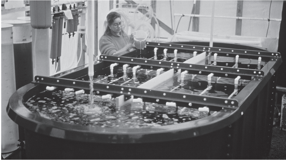
Figure 3. One of two 4,500 L fiberglass prototype raceway tanks for aquaculture of B. neritina , located within a nearshore greenhouse culture facility, Carlsbad, California. Technician is feeding one of various cultured micro-algal species grown in the “Sun-Tubes” at the left of the raceway.
