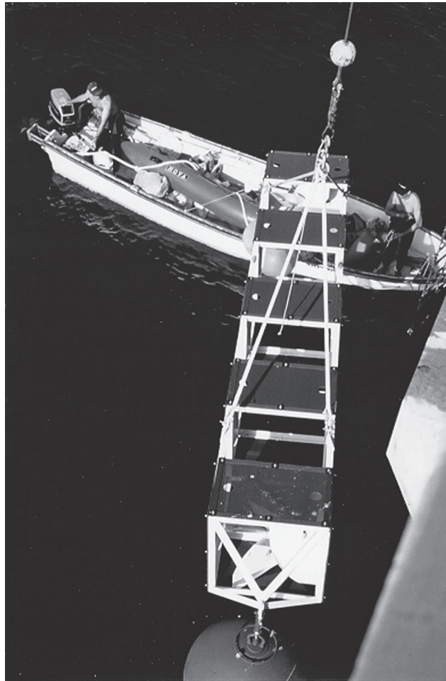
Figure 5. Launching of the 7-m long prototype in-sea aquaculture structure from the pier at UCSD Scripps Institution of Oceanography, La Jolla, California. Picture shows new, grey perforated pvc-plastic culture panels, large floatation sphere, and fixed-pitch propellers located within both ends of the structure.
