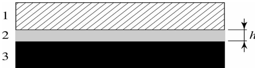
Figure 1 Definition of wetting film.
