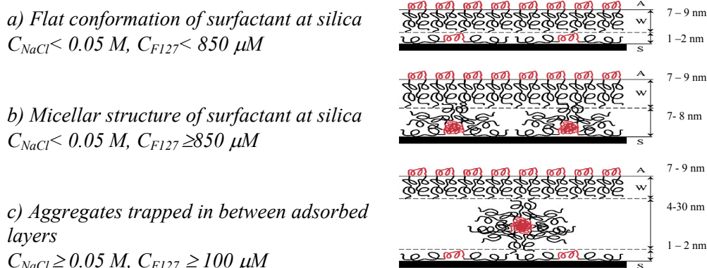
Figure 13 Possible structures of asymmetric liquid films stabilized by surfactant.
