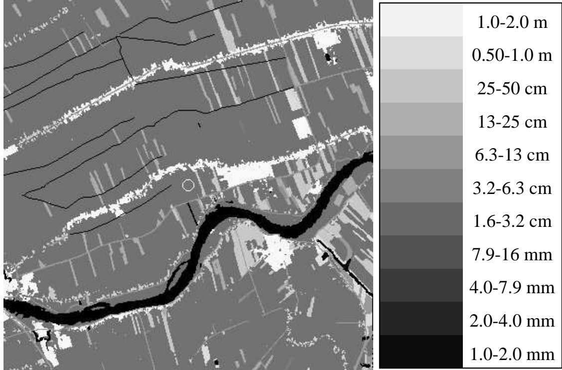
Figure 3.1: Roughness lengths in gray scale for the Cabauw environment [(10 \text{ km})^2] . The circle in the center of the figure indicates the tower position. Pixel size (25 \text{ m})^2 .
