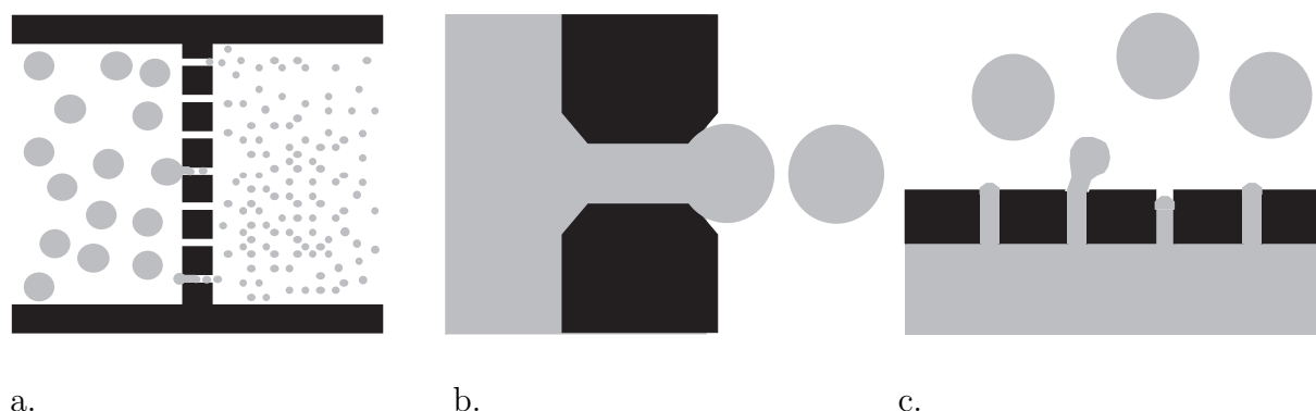
Figure 1.1: Overview of different methods of membrane emulsification: pre-mix membrane emulsification (a), microchannel emulsification (b), and cross-flow membrane emulsification (c).
