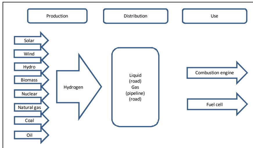
Figure 1 The hydrogen use chain: from well to wheel. Following <sup>21</sup>.
