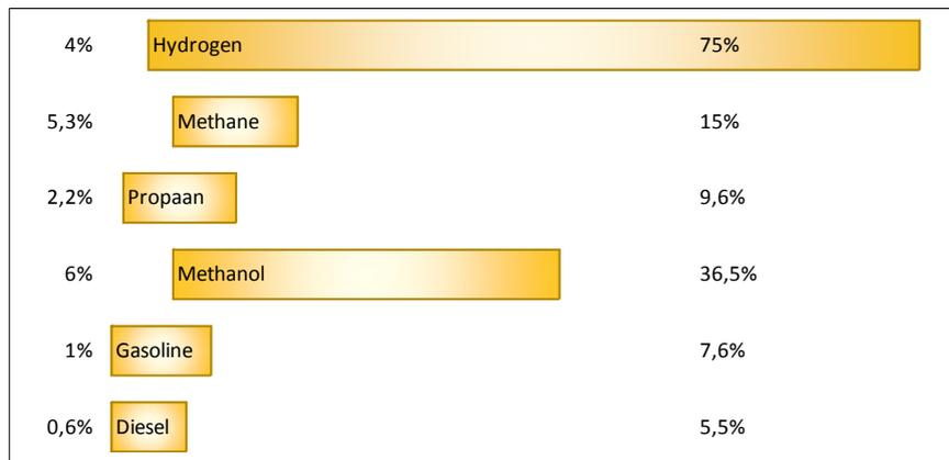
Figure 4 Inflammability ranges of fuel-air mixtures under normal temperature and pressure.<sup>77</sup>
