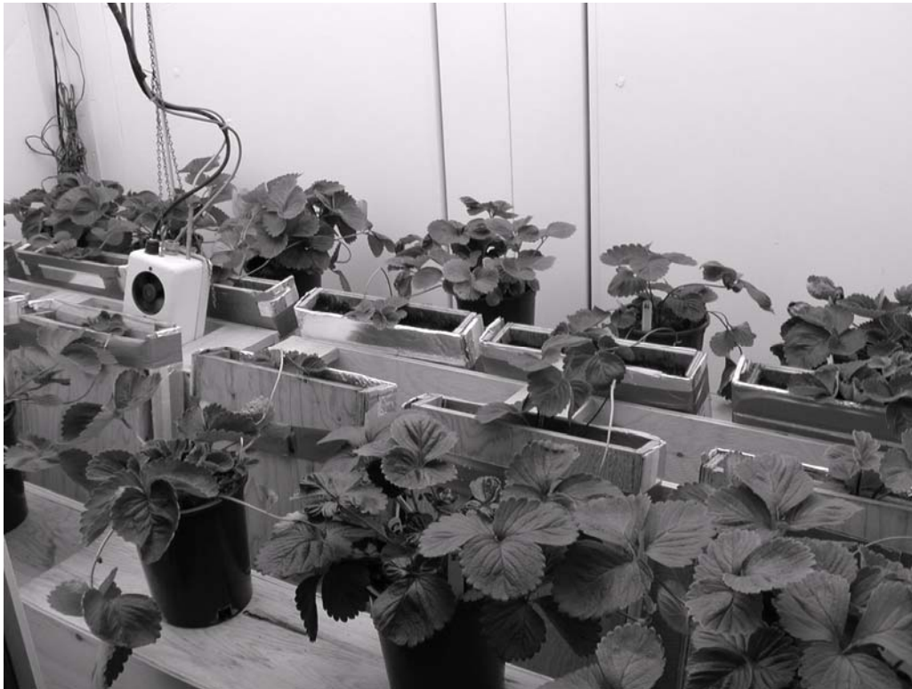
Figure 1. Each rhizotron unit was set on a wooden stand at a standard 15^\circ angle from the vertical inside the controlled environment growth chambers.
