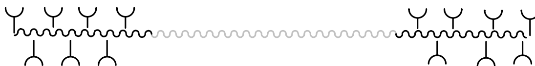
Figure 4: Schematic representation of block-copolymer, with ethylene oxide block in the middle and ligand group rich blocks at the ends.
