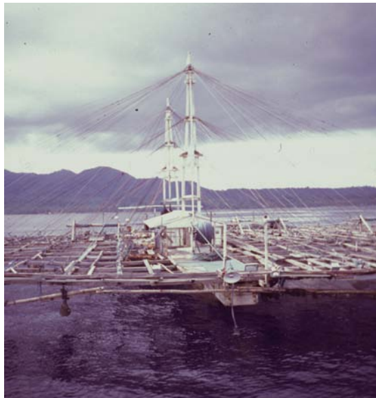
Picture 3: Liftnet platform, used in the coastal waters around Ambon and the Lease Islands.
