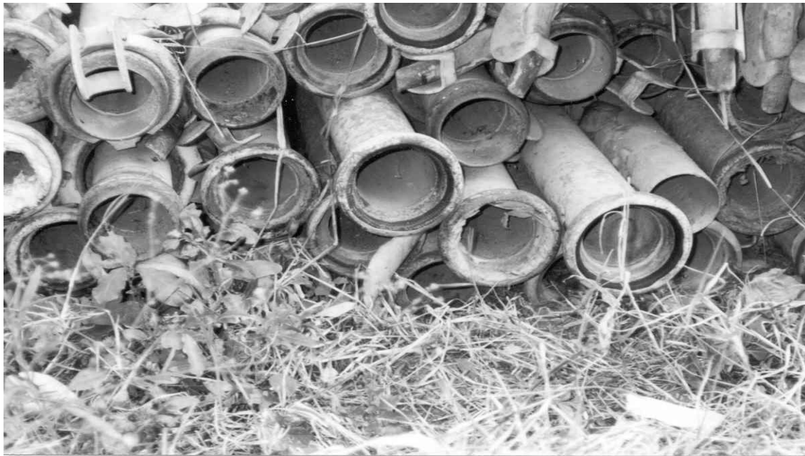
Photo 5.7.3 Local plastic and rubber used to seal GI couplings for the old pipes
