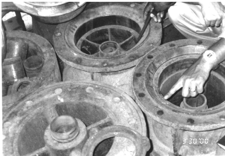
Photo 7.5.3 The Bonde pump wearing accelerated by sand in water
