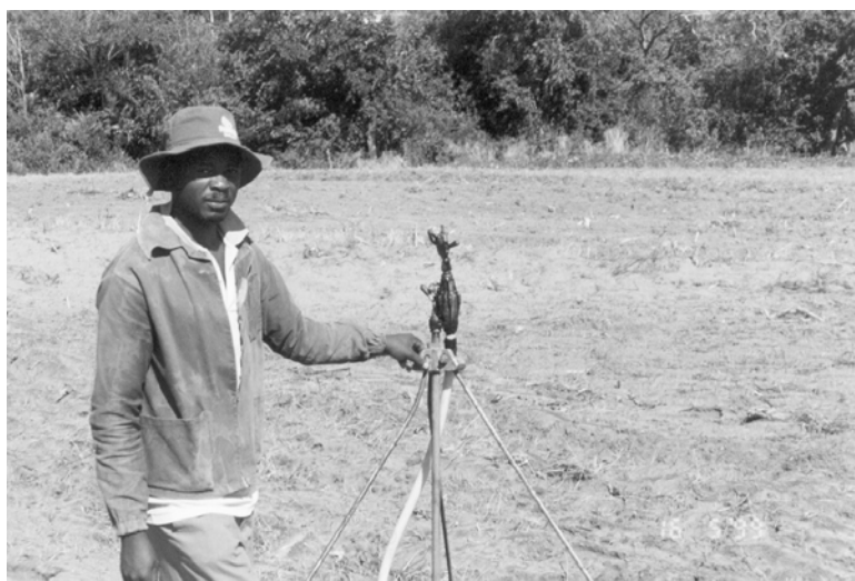
Photo 8.7.1 A pressure regulator “scud” directly connected to the sprinkler and hose to avoid damage at Mpudzi
