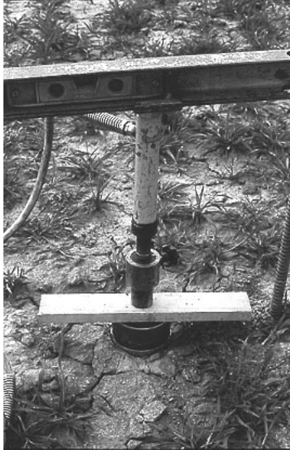
Figure 2.2 Taking samples of the top layer of a winter-wheat field, using hydraulic sampling equipment.
