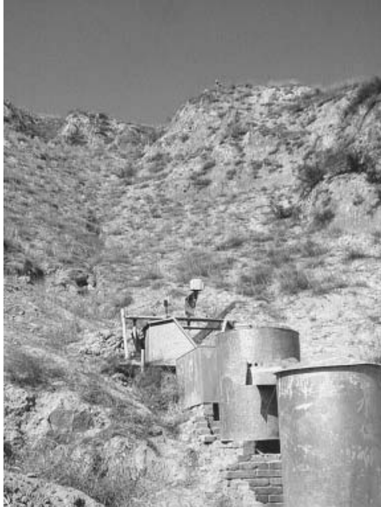
Figure 5.2 Flume at the outlet of the gully catchment to measure discharge and soil loss
