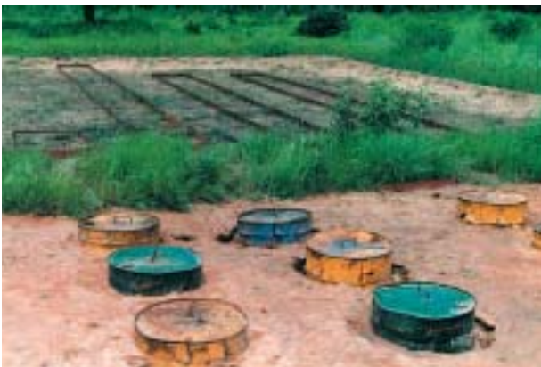
Runoff plots with different slope lengths and collection tanks
