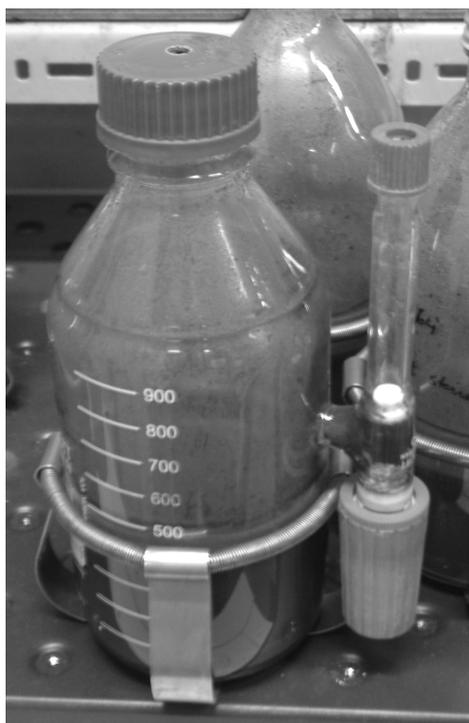
**Figure 2-2:** SPME batch reactor
