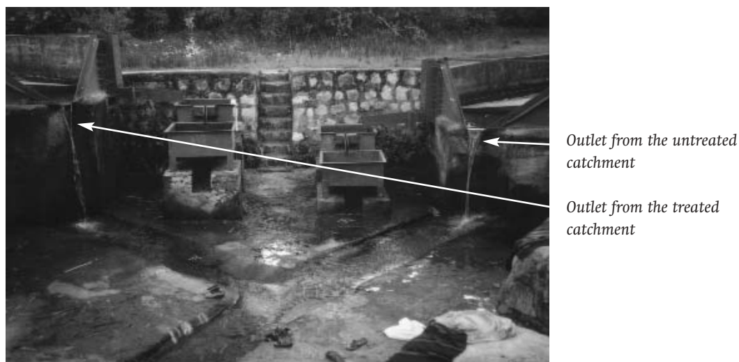
Plate 6.2: Hydrometric station at Gunno, Wolaita
