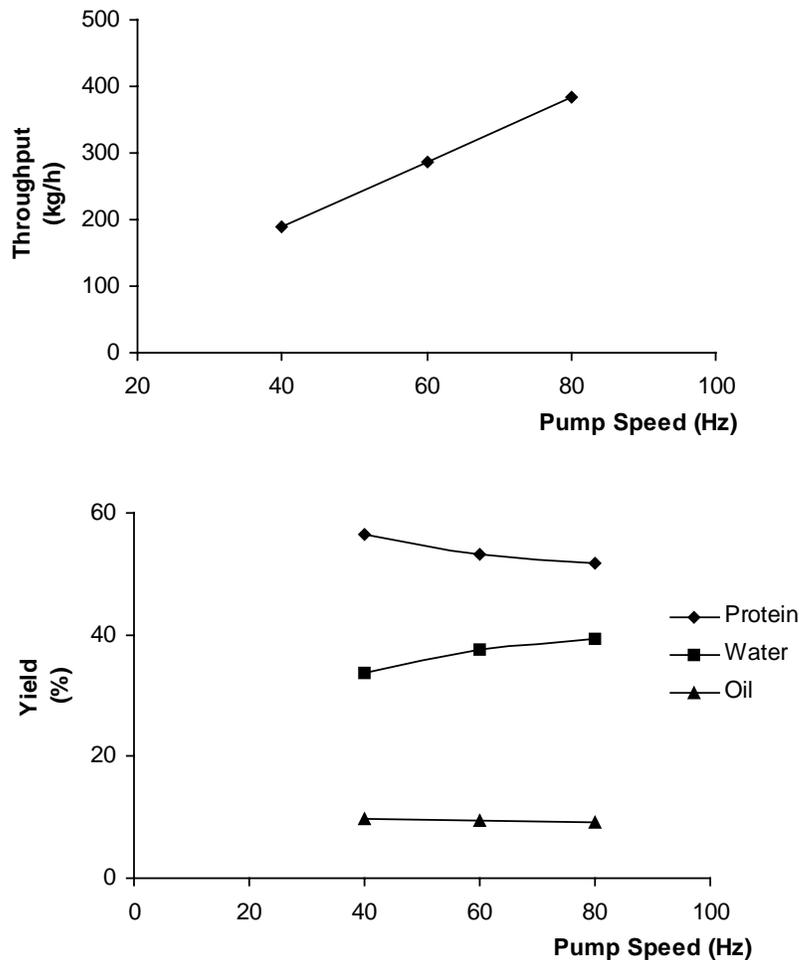
**Figure 1**– Variation of the total throughput and yield between mono pump speeds and quantity responses.
