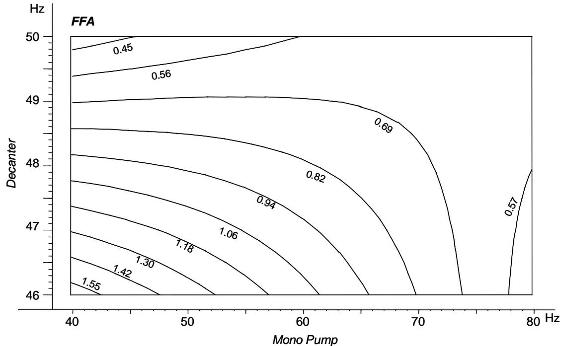
**Figure 3-** Contour plots for the effect of mono-pump and decanter speed on PV, Totox and FFA content of the extracted crude oil from herring byproducts during the process optimization experiment. The plots illustrate where in the experimental domain the lowest values could be obtained.
