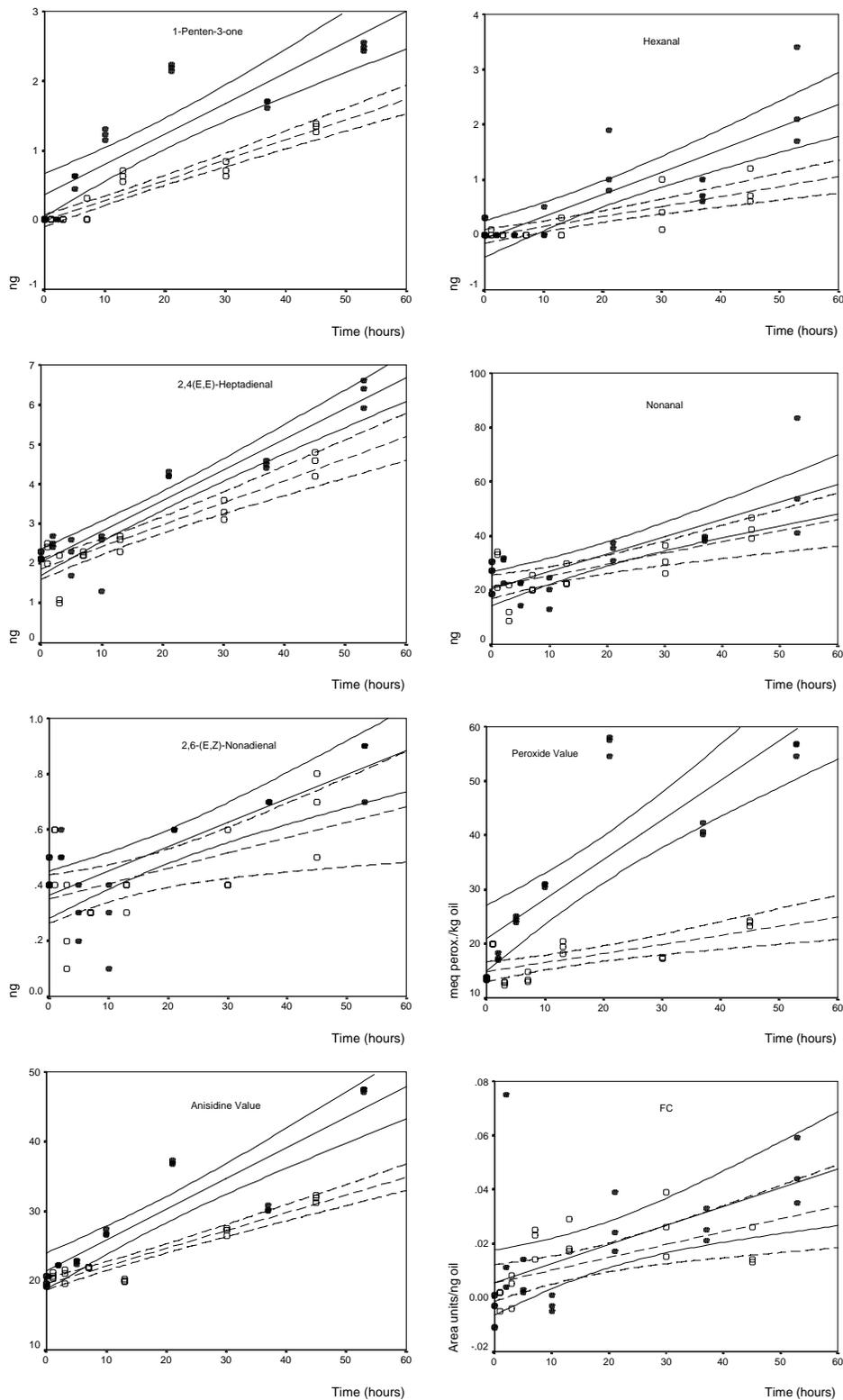
**Figure 2-** Linear regression lines, of the different lipid oxidation measurements, illustrating the change in (--- and  $\square$ ) = oil sampled after first oxygen exposure, and (— and  $\blacksquare$ ) = oil after a second oxygen exposure. Models describing these lines are shown in Table 1. The confidence bands are based on  $p = 0.05$ .
