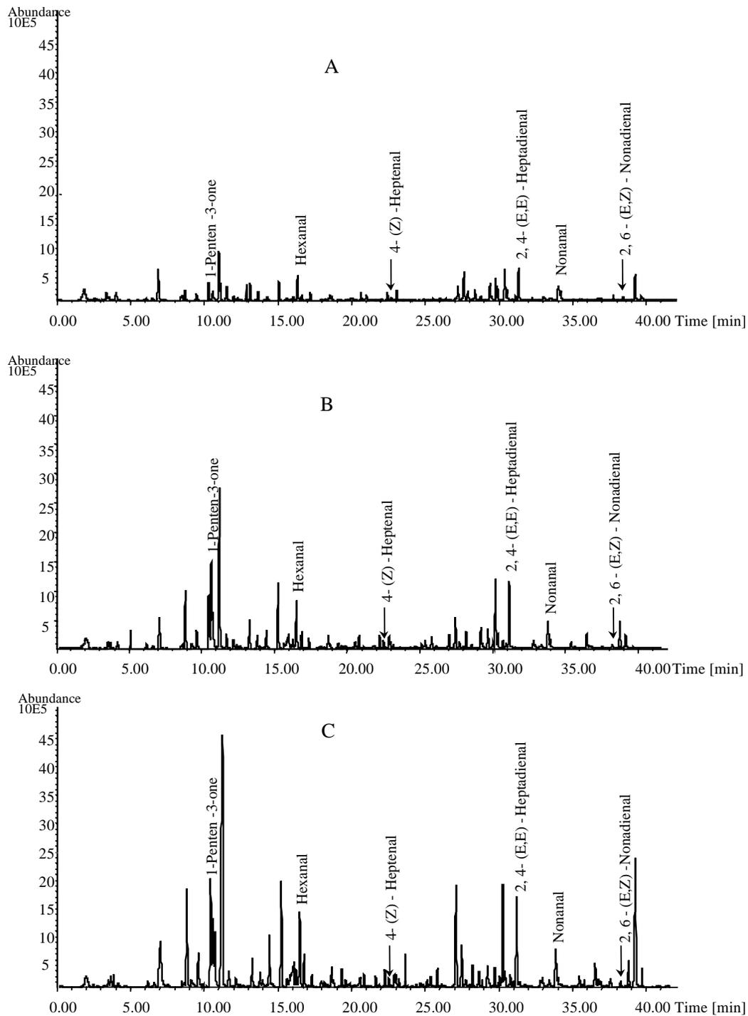
**Figure 1-** TIC (total ion current) chromatograms (0 – 42 min) for volatiles of crude fish oil produced from herring byproducts: (A) initial oil; (B) oil after 45 hours of accelerated oxidation at 50 °C in oxygen atmosphere (closed vessel with a volume oxygen/oil ratio of 1.3); (C) oil after 53 hours of oxidation at 50 °C after renewed oxygen supply (closed vessel with a volume oxygen/oil ratio of 3.5).
