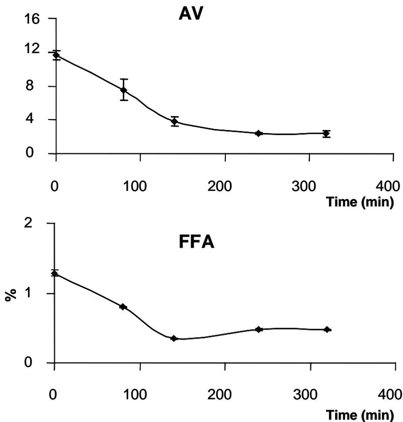
Figure 2- AV and FFA values of the crude herring oil for the reference points produced over time.
