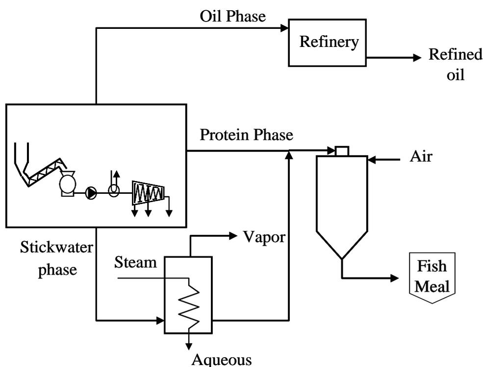
**Figure 4-** Flow diagram of a complete fish meal plant.
