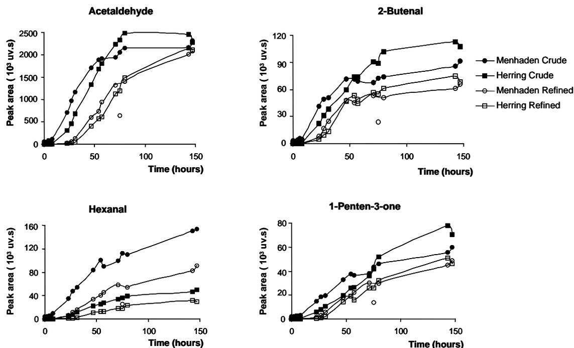
**Figure 4-** Oxidative stability of crude and refined herring and menhaden oil, when stored at 60 °C.
