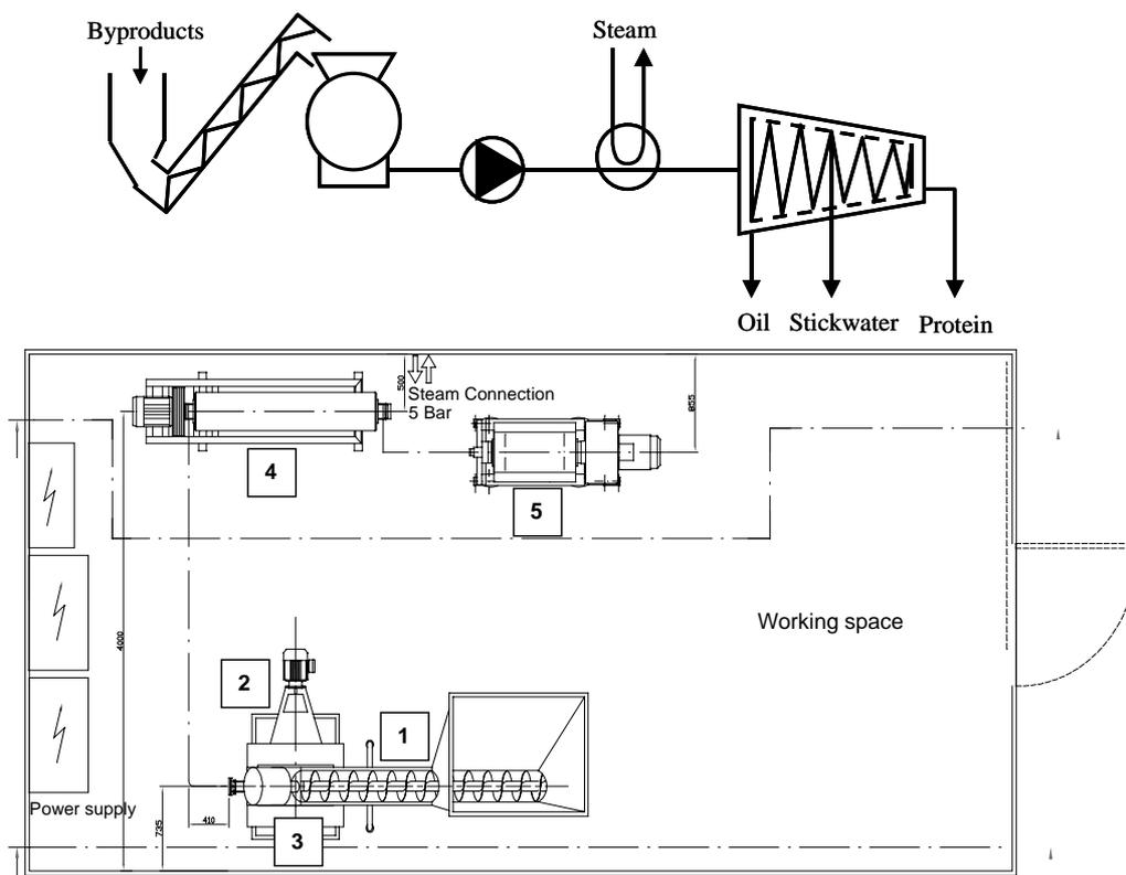
**Figure 3-** Layout of the pilot plant used for fish oil extraction process. 1: storage bin with feedscrew, 2: mincer, 3: mono-pump, 4: heat exchanger and 5: Decanter.
