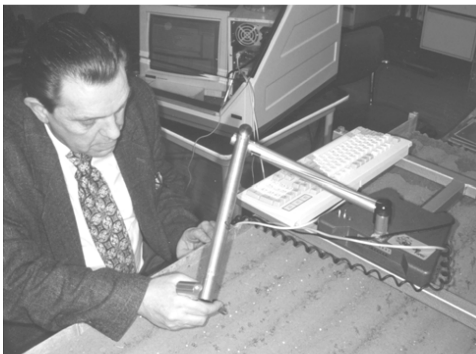
Fig. 4.2 Plant positions after harrowing are digitized using the SpaceArm™.
