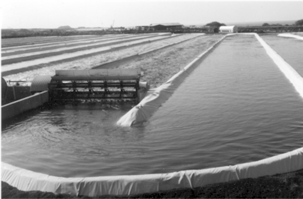
Figure 1.10. Shallow open raceway pond (Courtesy of Cyanotech Inc., Hawaii, USA).
