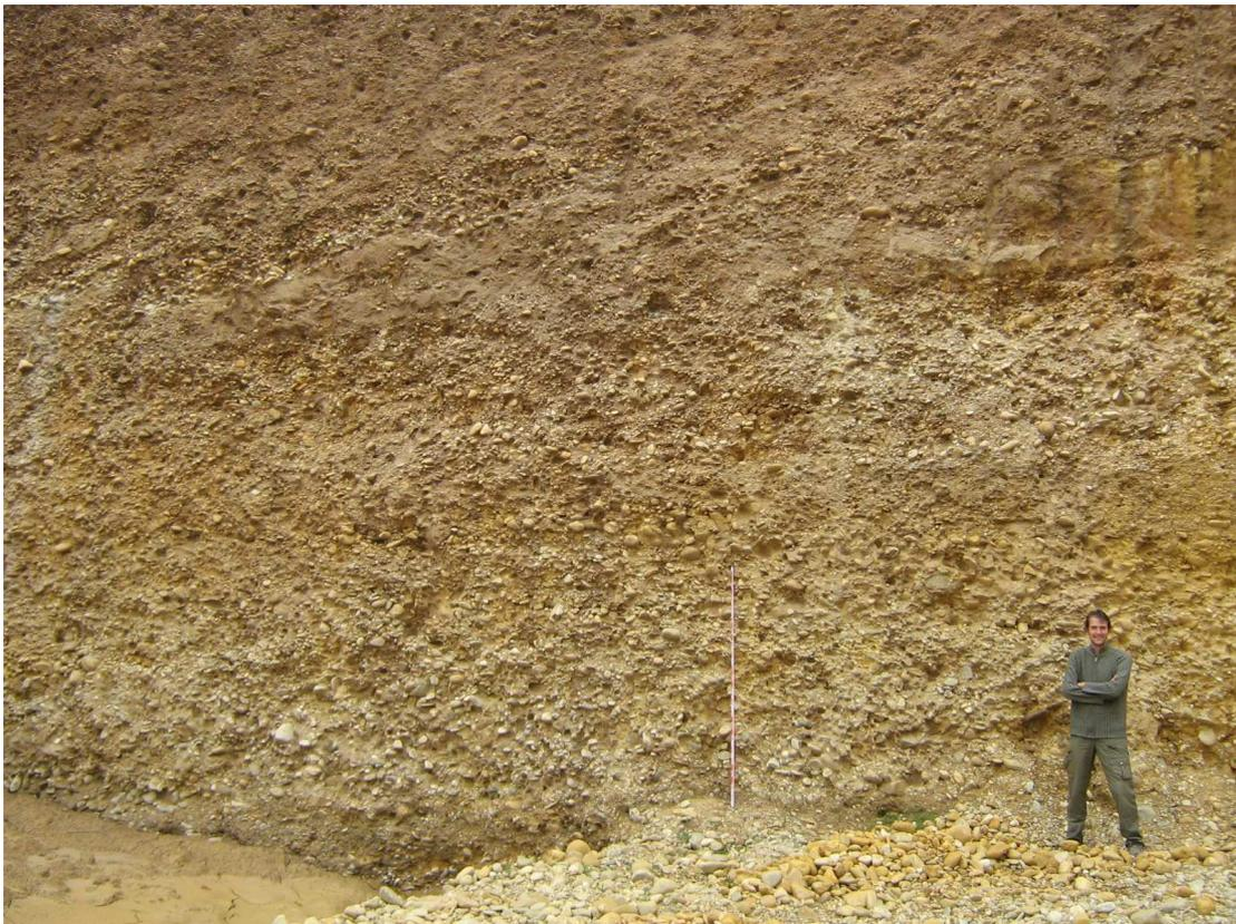
*Plate 10. T7. Quarry Chan de Vide, Galicia. Predominantly sandstone and quartz(ite) conglomerates in a clayey to loamy matrix. Measuring rod is 2 m high.*
