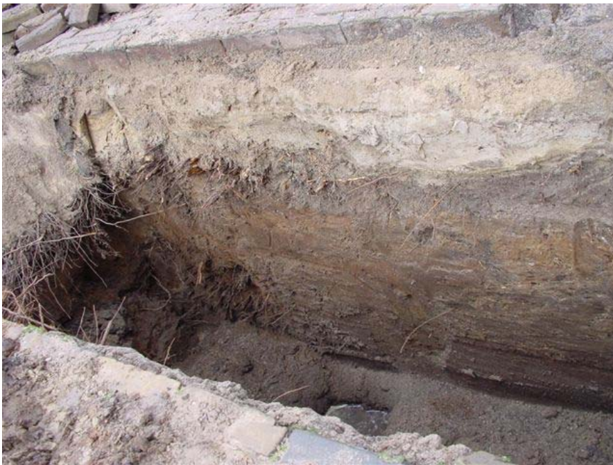
Figure 18 Layering of soil profile of root zone of tree no. 43 and groundwater table
