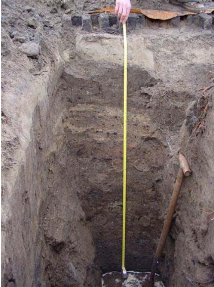
Figure 19 Taking undisturbed core samples at 3 depths on February 21, 2007. Six metal cylinders can be seen in the wall of the pit
