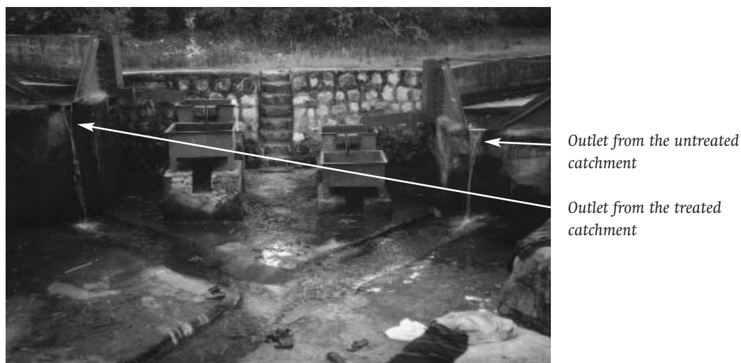
Plate 6.2: Hydrometric station at Gunno, Wolaita
