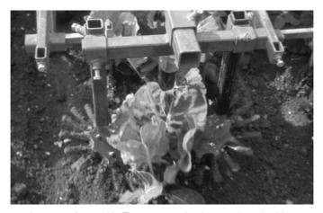
**Fig. 8.10.** Finger weeders, manufactured in Europe, operating in transplanted cabbages. (Photo by Wageningen UR Applied Plant Research.)
