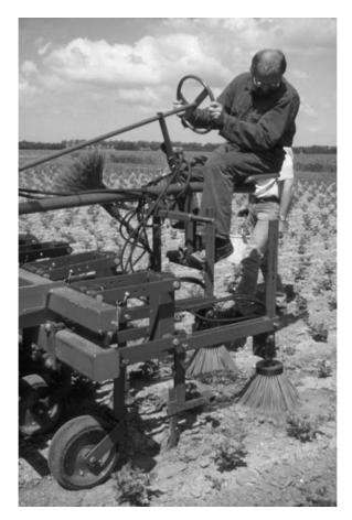
Fig. 8.7. Vertical axis brush weeder. (Photo by Wageningen UR Applied Plant Research.)
