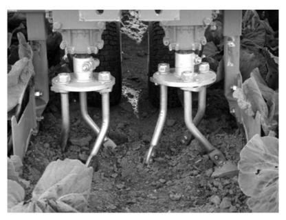
**Fig. 8.8.** Photo of the Weed-Fix cultivator, a vertical-axis rotary cultivator. (Photo by Wageningen UR Applied Plant Research.)
