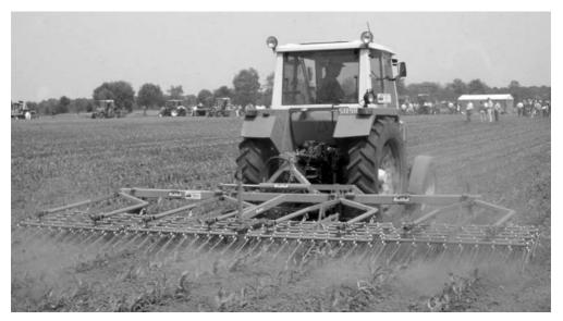
Fig. 8.4. Flex-tine harrow in silage maize. (Photo by Wageningen UR Applied Plant Research.)
