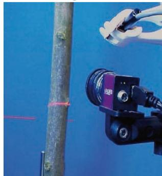
In laser triangulation, a moving laser line or a laser grid is combined with a camera. A camera 'looks' at an object from an angle in relation to the laser and 'sees' a height profile. A height profile can be distilled from this action. By using several cameras and lasers from different angles, a complete 3D image can be created.
