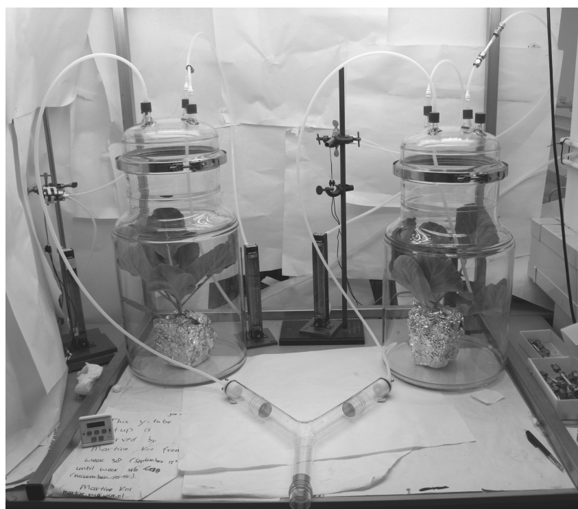
Figure 1. The experimental set up for preference testing and volatile trapping
