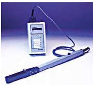
Figure 3.2: LAI-2000 instrument.
