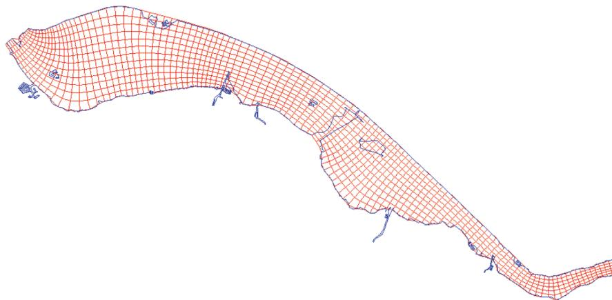
FIGURE 2.2 HYDRODYNAMIC GRID SCHEMATISATION FOR (A) DELTSE HOUT AND (B) THE EXISTING GRID FOR GOIMEER-EEMMEER
