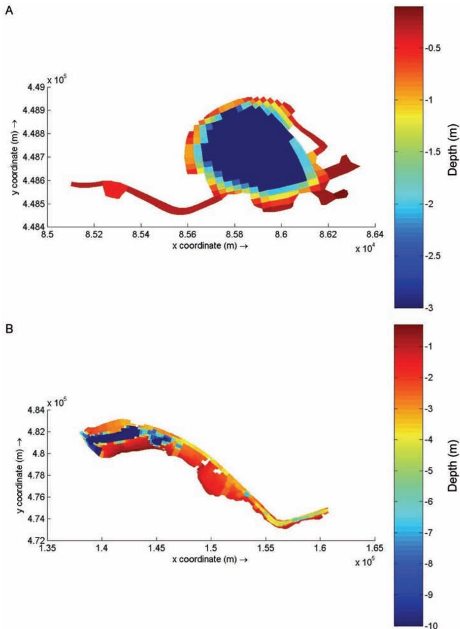
FIGURE 2.7 HYDRODYNAMIC MODEL BATHYMETRY FOR (A) SLOTERPLAS AND (B) WESTEINDERPlassen
