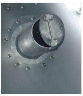
A deflector prevents feed from separation in small and large particles.
