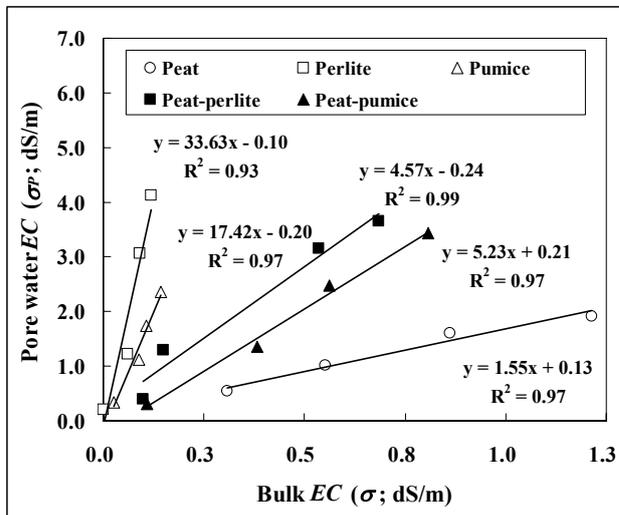
Fig. 3. The relationship between bulk EC ( $\sigma$ , as measured by means of WET<sup>®</sup> sensor) and pore water EC ( $\sigma_p$ ) in different horticultural substrates.
