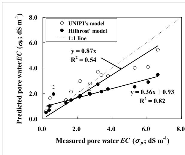
Fig. 6. The relationship between measured and predicted values of pore water EC ( $\sigma_p$ ) in a peat-pumice mixture irrigated to container water capacity with nutrient solution of different salinity (EC) and then dried in air to desired volumetric water content ( $\theta$ ). The EC was measured in the water collected by centrifugation or calculated from the bulk EC ( $\epsilon$ ) provided by WET<sup>®</sup> sensor using two different equations (see text for details).
