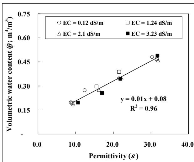
Fig. 4. The relationship between permittivity ( $\epsilon$ , as measured by means of WET<sup>®</sup> sensor) and volumetric water content ( $\theta$ ) in a peat-pumice mixture irrigated to container water capacity with nutrient solutions of different salinity (EC; the values are reported in the box).
