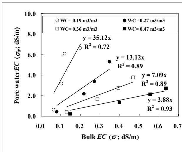
Fig. 5. The relationship between bulk EC ( $\sigma$ , as measured by means of WET<sup>®</sup> sensor) and pore water EC ( $\sigma_p$ ) in a peat-pumice mixture irrigated to container water capacity with nutrient solutions of different salinity (EC; the values are reported in the box) and then dried in air to desired water content (WC).
