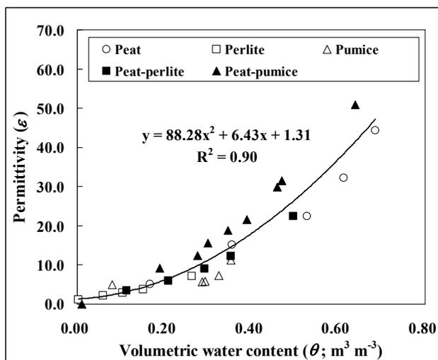
Fig. 1. The relationship between permittivity ( $\epsilon$ , as measured by means of WET<sup>®</sup> sensor) and volumetric water content ( $\theta$ ) in different horticultural substrates.
