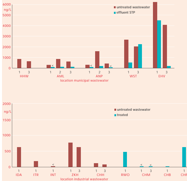
F 3.6 Occurrence of bisphenol-A in untreated municipal and industrial wastewater and effluent of biological treatment plants.
