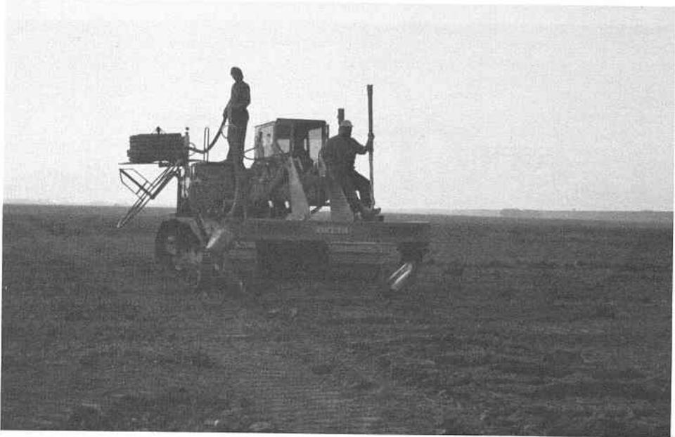
Figure 5 Trenchless drainage machine 'delta plough' installing prewrapped corrugated pvc pipe in The Netherlands. Maximum installation depth 1.8 m
