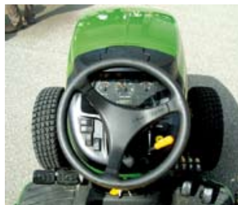
Dashboard van de 3720. Knop LoadMatch, handgas, aftakasknop.
