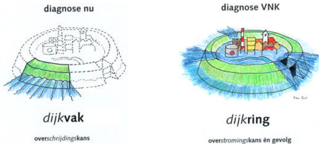
Fig. 1: Left: approach for a section of the ring, right: 'total ring approach' used in FLORIS (VNK)
