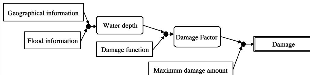
*Fig. 8: Steps for damage computation*
