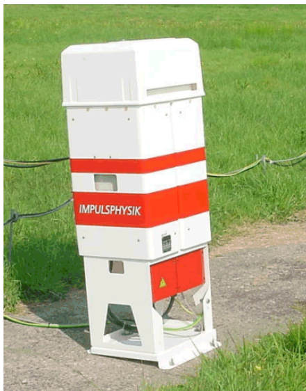
FIGURE 3.1. Left: The Vaisala-Impulsphysik LD-40 ceilometer, mounted on a concrete base. Right: Schematic overview of operation of the LD-40, with: cpu (CPU), det (detector), las (laser), tes (test laser), wbs (detector for window backscatter), ref (reference detector). Adapted from Wauben et al. (2001).
