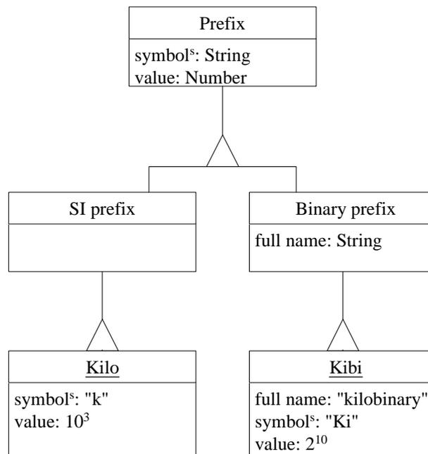
Fig. 5. Class diagram of the concept *prefix*.
