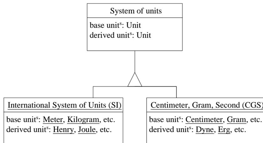
**Fig. 8.** Class diagram of the concept *system of units*.
