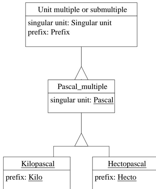
Fig. 6. Class diagram of the concept *unit multiple or submultiple*.
