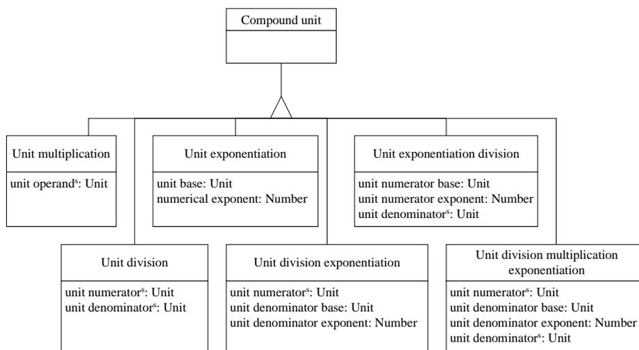
**Fig. 7.** Class diagram of the concept *compound unit*.
