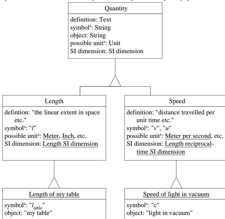
**Fig. 2.** Class diagram of the concept *quantity*.
