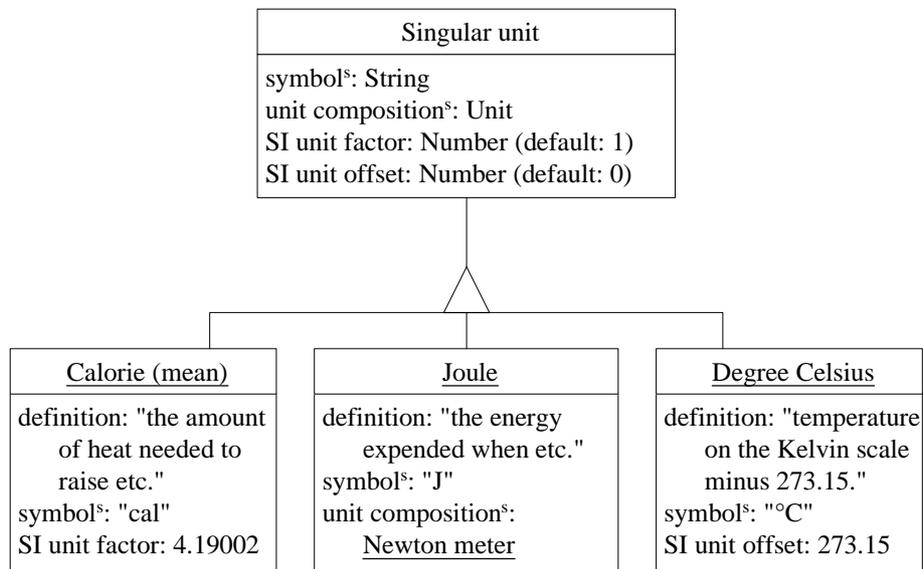
Fig. 4. Class diagram of the concept *singular unit*.
