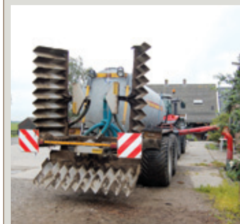
In transport is de bemester 2,30 meter breed.
