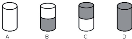
Figure 1. Experimental design of the four artificial soil profiles a , profile of 0-10 cm reference soil; b , profile of reference topsoil 0-5 cm and contaminated sub-layer 5-10 cm; c , profile contaminated topsoil 0-5 cm over a reference sub-layer 5-10 cm and; d , profile of 0-10 cm contaminated soil.
