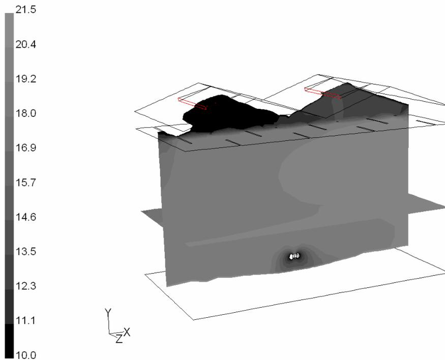
Fig. 7. Temperature (left) and relative humidity distribution at a height of 2 meter when the forced air flow is  $1.7 \text{ m}^3 \text{ m}^{-2} \text{ uur}^{-1}$  with a temperature of  $5^\circ\text{C}$  and a relative humidity of 95%.
