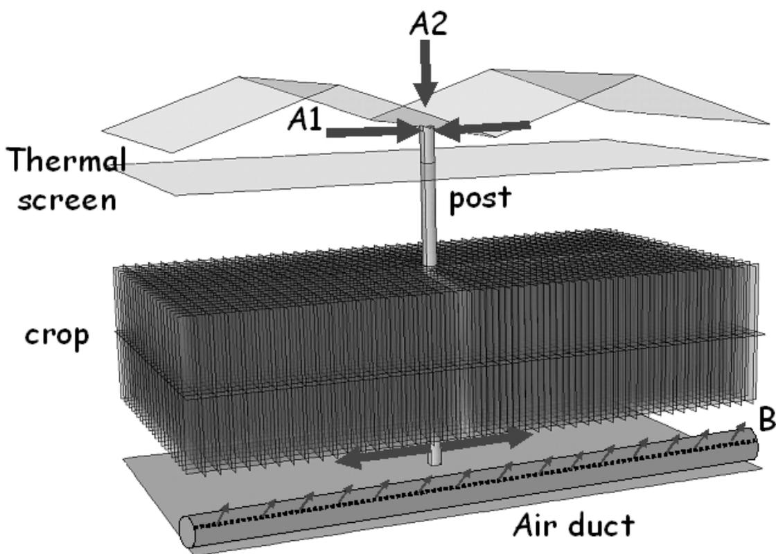
Fig. 1. A schematic representation of the system where A1 and A2 locally ventilated air for above the screen or for outside and system B where the air distributed by a air duct.
