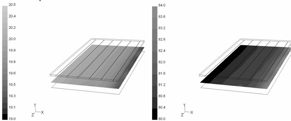
Fig. 5. Temperature (left) and relative humidity distribution at a height of 2 meter after 3 minutes when the openings in between the thermal screen is 10 cm.
