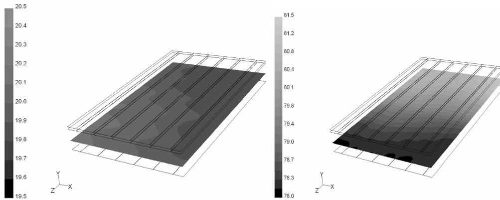
Fig. 6. Temperature (left) and relative humidity distribution at a height of 2 meter when the forced air flow is  $1.7 \text{ m}^3 \text{ m}^{-2} \text{ uur}^{-1}$  with a temperature of  $5^\circ\text{C}$  and a relative humidity of 95%.
