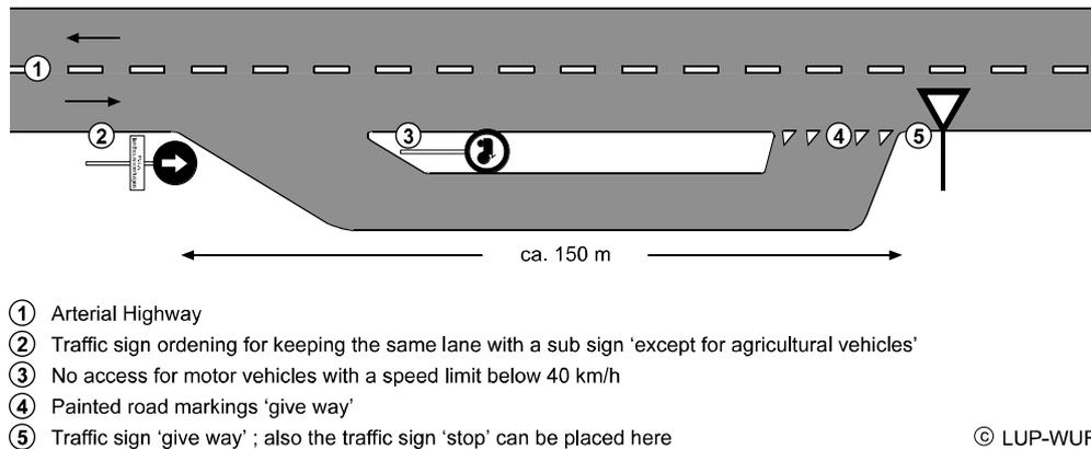
Figure 2. A rough sketch of a passing bay for agricultural vehicles alongside an arterial highway (Jaarsma *et al.* 2005)
