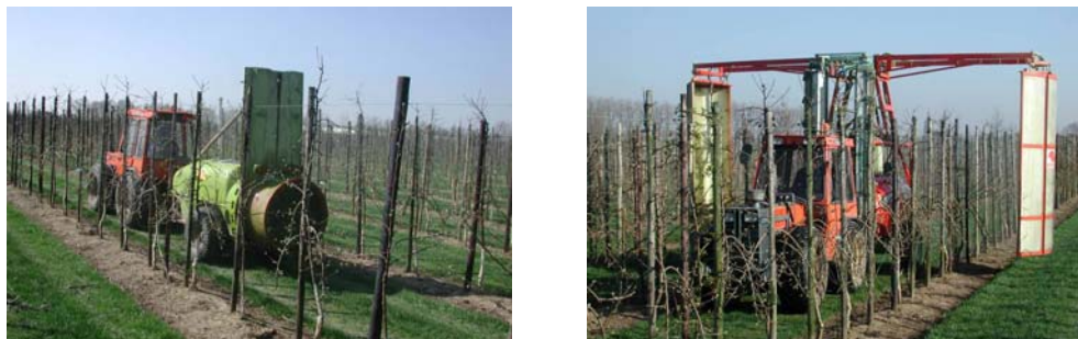
Figure 1a. Reference cross flow spraying machine (Munckhof) and Wanner sprayer with reflection shields.
