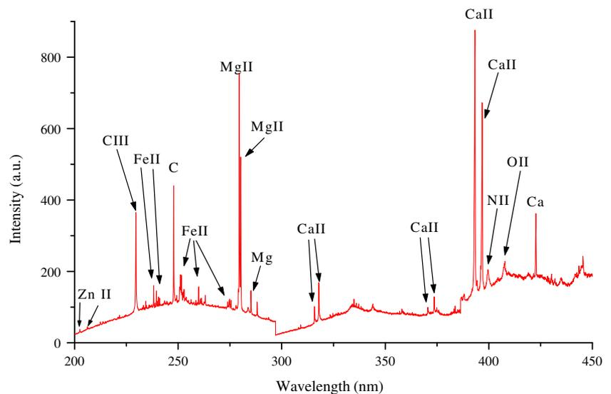
**Fig. 3** Laser-induced breakdown spectra of *T. dioica* in the spectral range 200–900 nm
