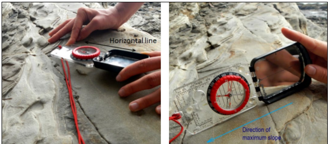
Figure 9 Method of measuring the bedding (left) and the dip angle (right). (Taken from Physical Geology by Steven Earle, chapter 12.4 - figure 12.19)
