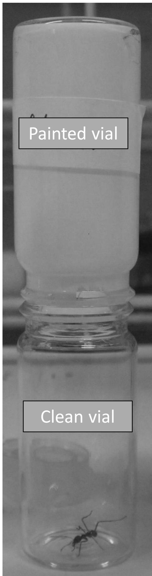
Fig. 9. Double-vial set-up to test the particle detachment hypothesis after contamination of feet of *A. cephalotes* ants: the top vial was painted with test paint and the bottom vial was clean glass.
