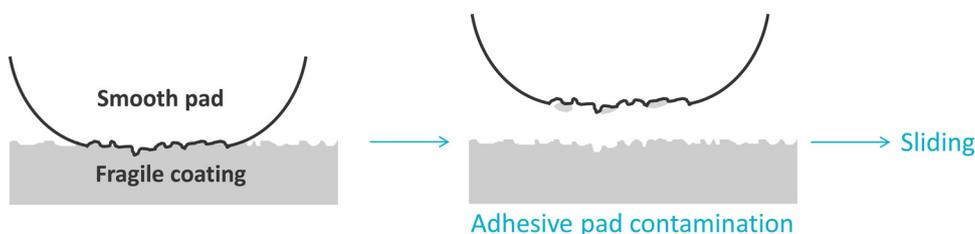
Fig. 1. Schematic showing the contamination mechanism of smooth adhesive pads on slippery, fragile surfaces.
