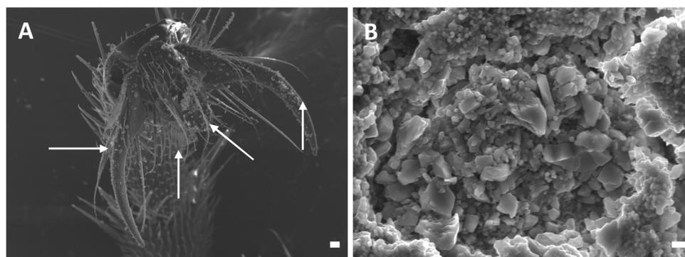
**Fig. 10.** SEM images of (A) contaminated *A. cephalotes* tarsus after climbing a scrubbed paint panel. Arrows show contaminating particles. (B) exposed “craters” in loose particles after the coating was scrubbed for 2000 cycles. Scale bars: (A) 10  $\mu$ m and (B) 1  $\mu$ m.
