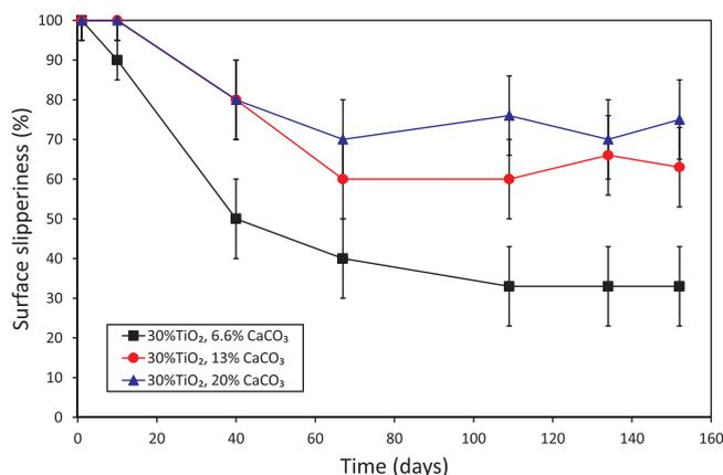
**Fig. 11.** Long-term slipperiness test: slipperiness (portion of unsuccessful ants) measured as a function of time during 5 months by leaving the painted panels (30% TiO<sub>2</sub>, variable concentration of CaCO<sub>3</sub>) in the *A. cephalotes* colony's rearing. A slipperiness plateau was reached within ca. 2 months for the three paints, which suggests that thereafter, insect attachment forces were reduced through surface roughness.
