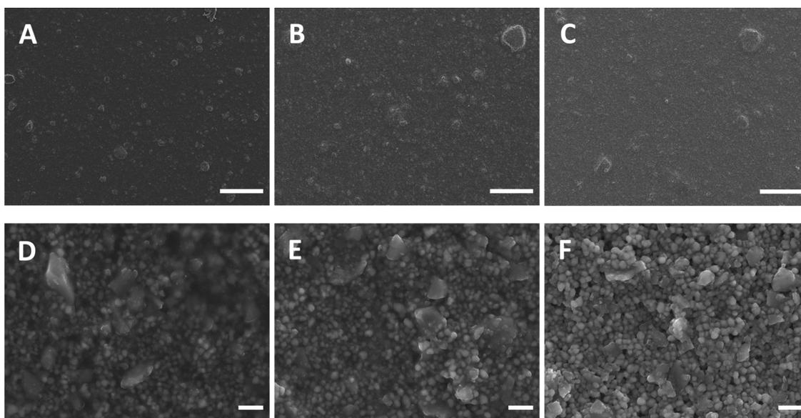
**Fig. 4.** SEM images of 30 wt% TiO<sub>2</sub>, 20 wt% CaCO<sub>3</sub> paint surfaces with varying PVC: (A, D) PVC 50, (B, E) PVC 60 and (C, F) PVC 70. Paints shown in (B, E) and (C, F) are formulated above their CPVC. Scale bars: (A–C) 100 μm and (D–F) 1 μm.
