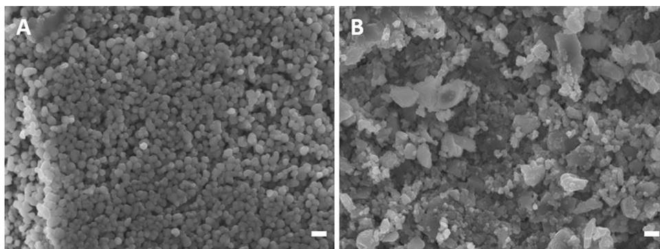
**Fig. 3.** SEM images of the (A) titanium dioxide (Tiona 595, spherical shape, mean diameter: 300 nm) and (B) calcium carbonate (Omyacoat 850-OG, platelet shape, mean diameter: 1  $\mu\text{m}$ ) grades used in this study. Scale bars: 1  $\mu\text{m}$ .
